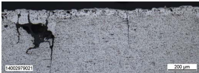
Fig. 5. Cross section after AC-3 endurance test
